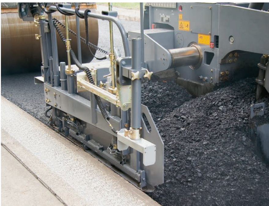
> Referencing from a tensioned wire with sonic grade sensor
