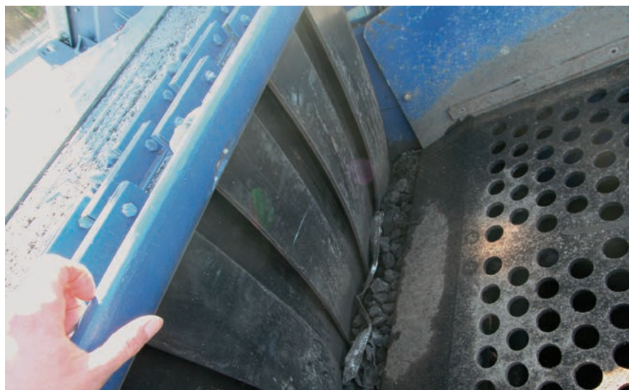
> Chains and rubber curtain in use in the MR 130 R EVO impact crusher
